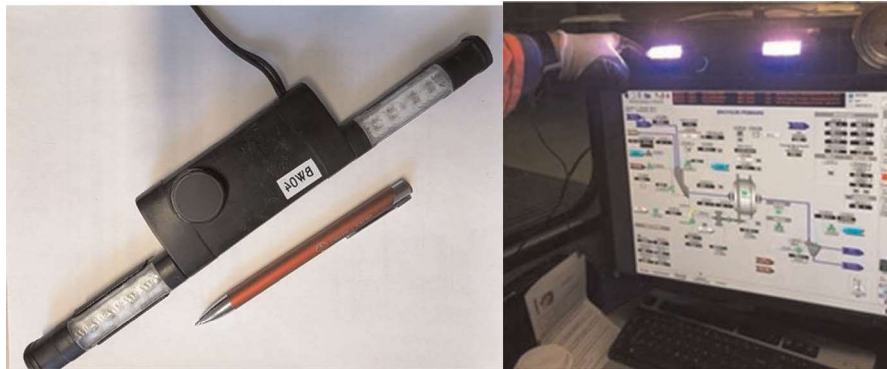
FIGURE 1. Pictures of the blue-enriched light custom-made device on the left, and when in use on the right.
